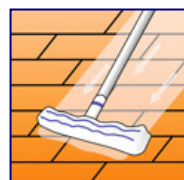
Generously apply Lithofin TC Classic Wax and allow to dry for 20-60 min.
